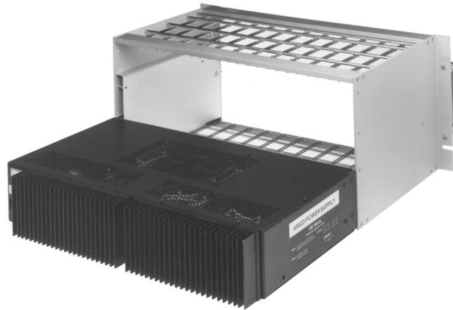
An external slide switch allows selection of either 115 or 220 V AC as the power input. By changing pins on an internal connector, this selection can be altered to 100 and 200 V AC. An international standard IEC power connector permits power cords and plugs that meet local electrical standards to be used for the input power. Control of the primary power is provided by the On/Off switch on the NIM bin control panel.
