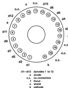
Fig. 2. Pin Assignments.
