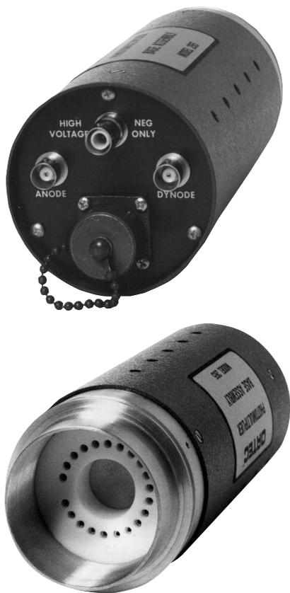
The ORTEC Model 265A Photomultiplier Base is a mechanical assembly and a resistive voltage divider network, with appropriate capacitive decoupling, for operation of 12-stage photomultiplier tubes (PMTs). It is particularly suited to applications requiring fast timing or single photon counting. The Model 265A accommodates the following types of PMTs.
