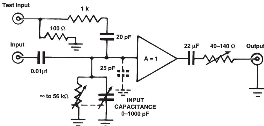
Fig. 1. Simplified Schematic of the Model 113.
