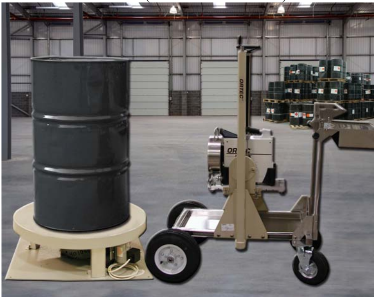
Figure 1. A measurement station using a trans-SPEC.
