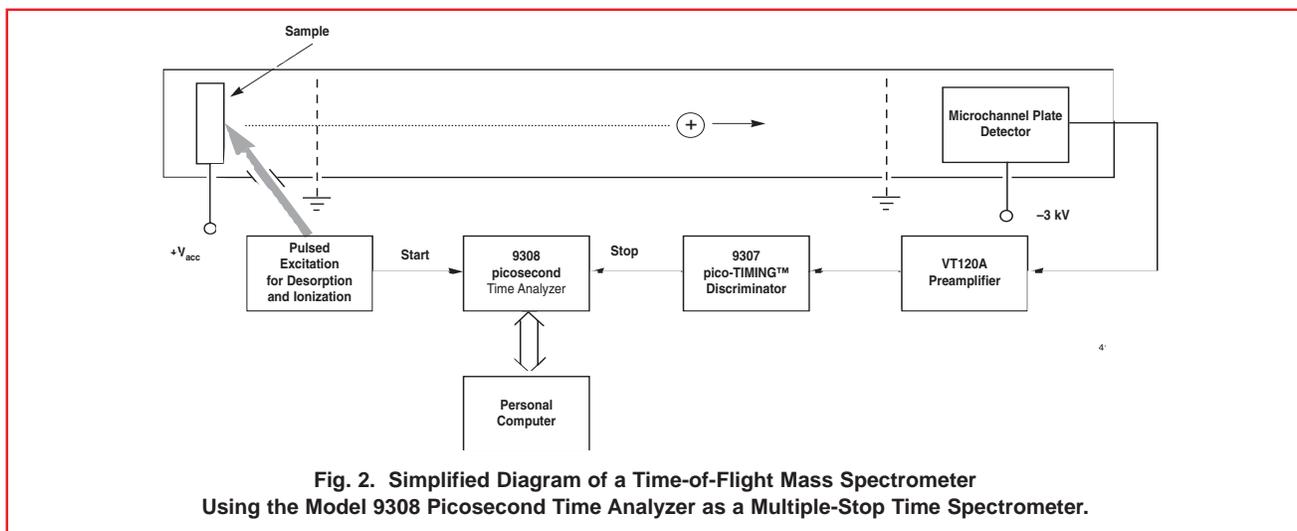
The high data rates permitted by the low end-of-pass dead time and the multiple-stop capability of the Picosecond Time Analyzer, together with the 65,536:1 time resolution, make the Model 9308 a particularly productive tool for time-of-flight mass spectrometry.
