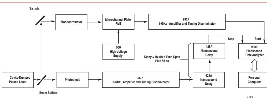
Fig. 6. The Reversed Start/Stop Arrangement for Fluorescence Lifetime Spectrometry.
