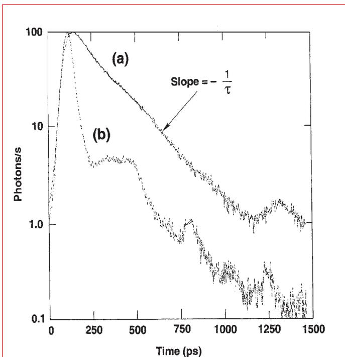
Fig. 5. (a) The Fluorescence Decay of Diphenylbutadiene in Butanol ( $\tau = 128$  ps). (b) The Instrument Response Function for  $\tau = 0$ . (Courtesy of Dr. John Kauffman, University of Missouri-Columbia.)
