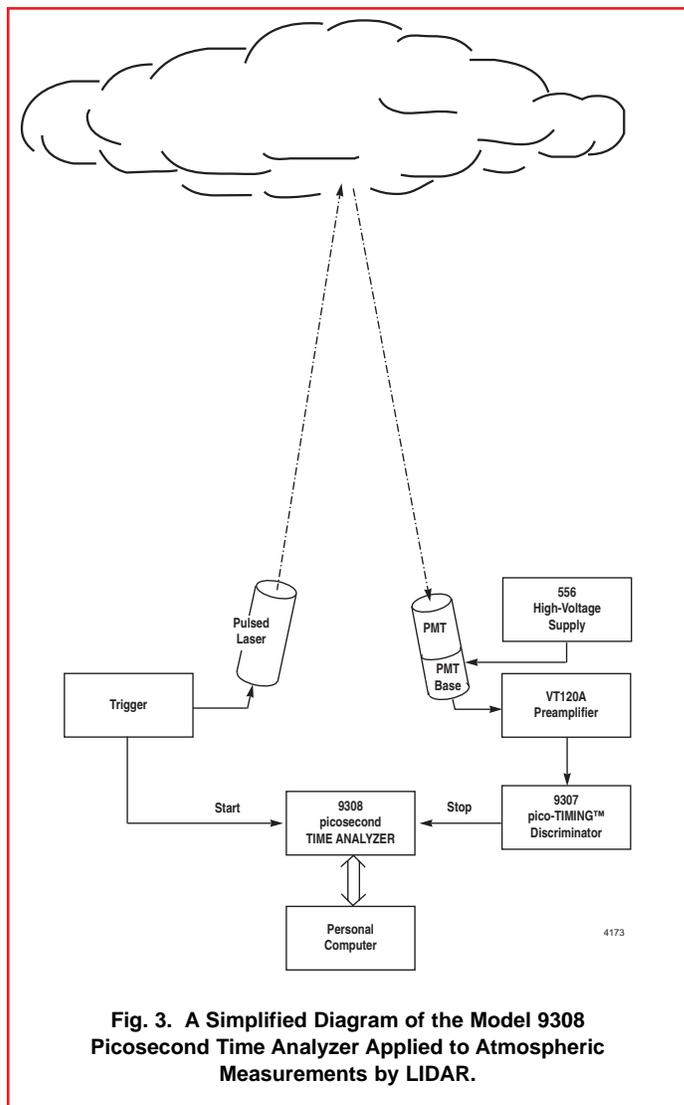
**Fig. 3. A Simplified Diagram of the Model 9308 Picosecond Time Analyzer Applied to Atmospheric Measurements by LIDAR.**
