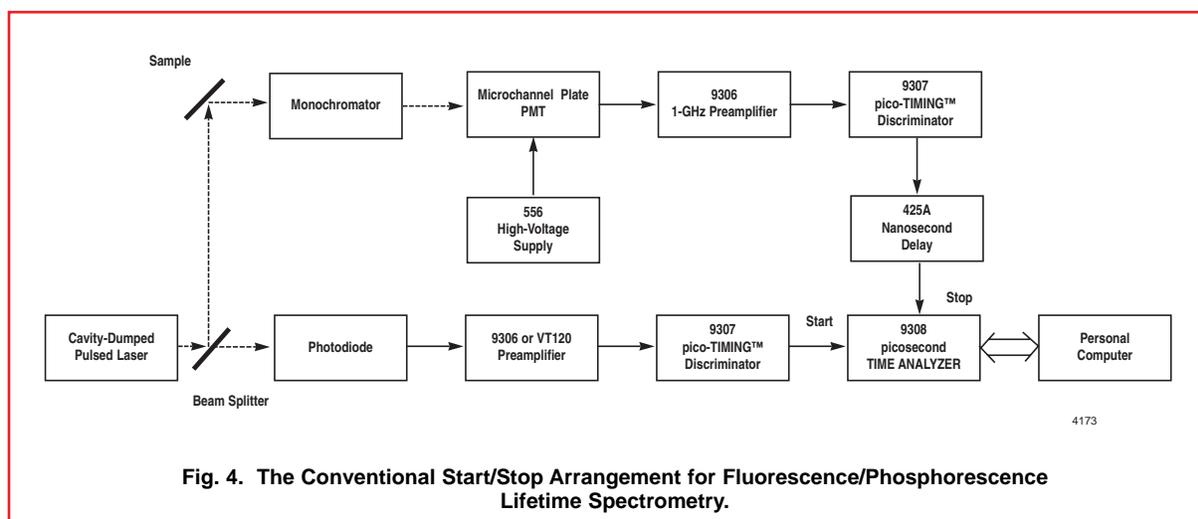
**Fig. 4. The Conventional Start/Stop Arrangement for Fluorescence/Phosphorescence Lifetime Spectrometry.**
