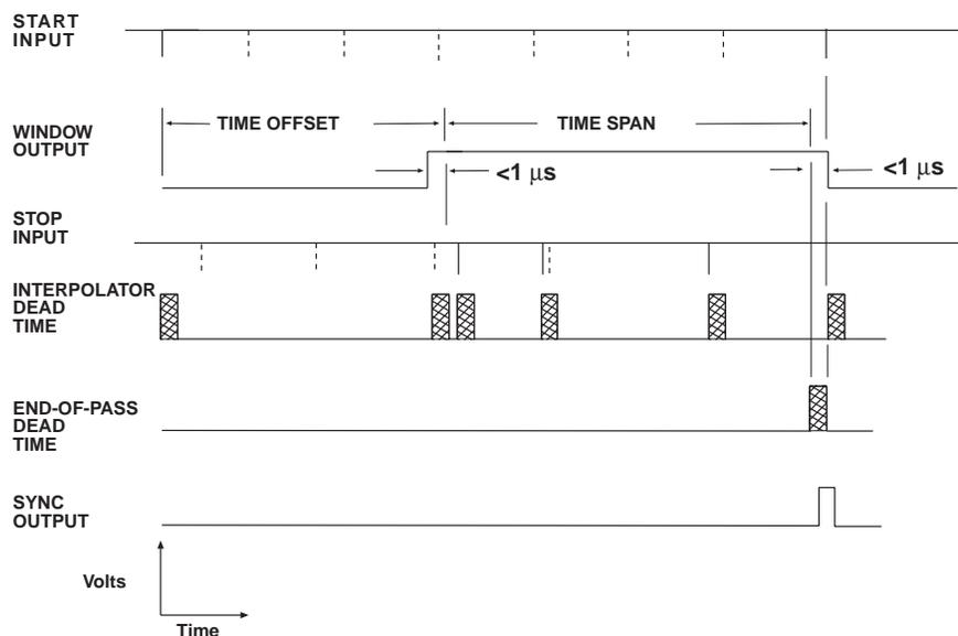
**Fig. 1. Timing Diagram for the Model 9308 Picosecond Time Analyzer.**
