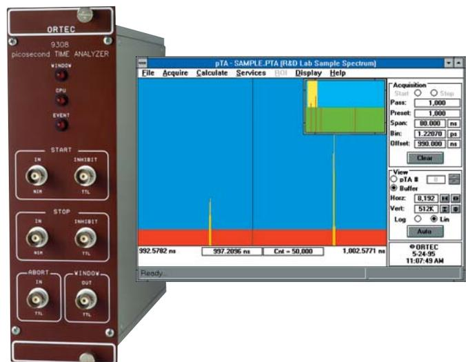
LASER operating at a 100-kHz repetition rate could be used to measure the distance to multiple objects located at distances ranging from 100 to 147 meters. Each LASER pulse starts a pass, and the photons reflected from the various objects generate the Stop pulses that arrive 667 to 980 ns after each LASER pulse. The arrival times of multiple Stop pulses can be recorded during each pass through the selected time range.
