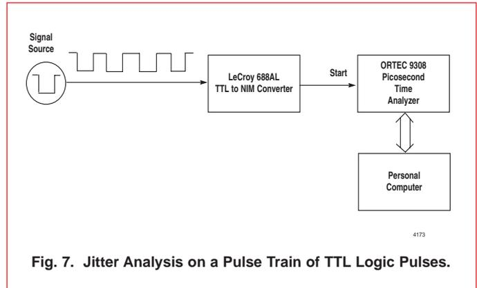
Fig. 7. Jitter Analysis on a Pulse Train of TTL Logic Pulses.
