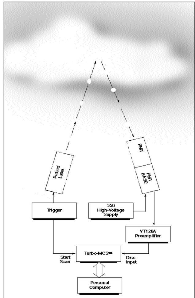
Fig. 7. A Simplified Diagram of the Application of Turbo-MCS™ to Atmospheric Measurements by LIDAR.
