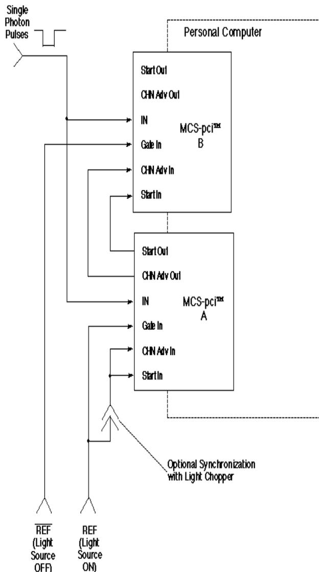
Fig. 4. Recording the Time Profiles for the Signal and Dark Counts (A) and the Dark Counts (B) Utilizing a Synchronized Pair of Multichannel Scalers for Single-Photon Counting.
