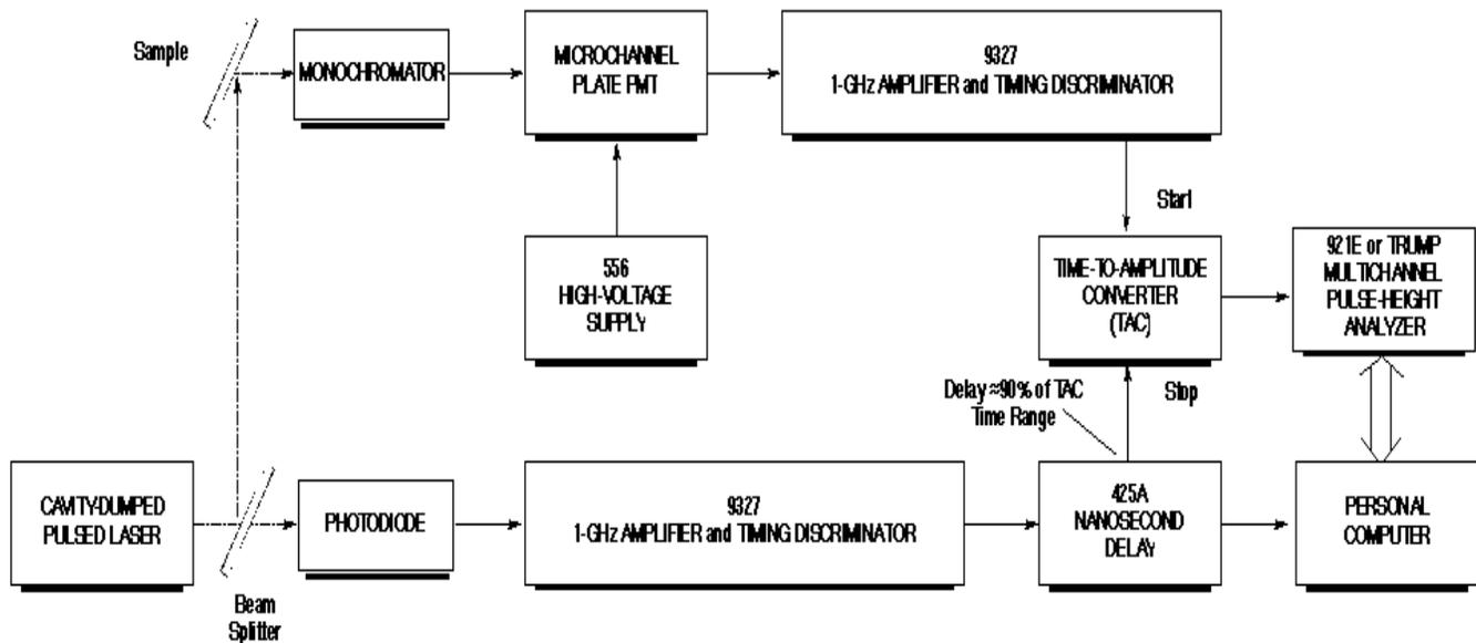
Fig. 6. Typical Block Diagram for a Fluorescence Lifetime Spectrometer.
