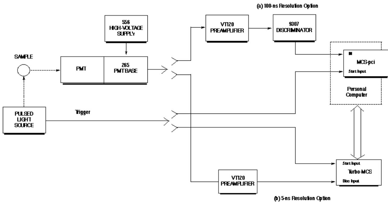
Fig. 5. Time-Correlated Single-Photon Counting with a Pulsed Light Source.
