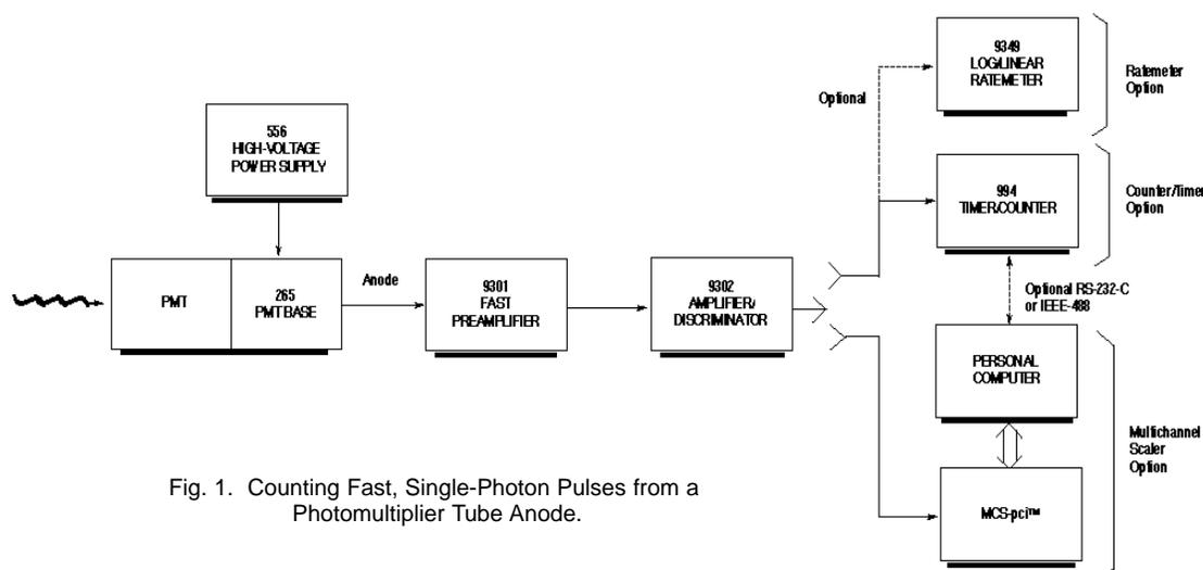
Fig. 1. Counting Fast, Single-Photon Pulses from a Photomultiplier Tube Anode.
