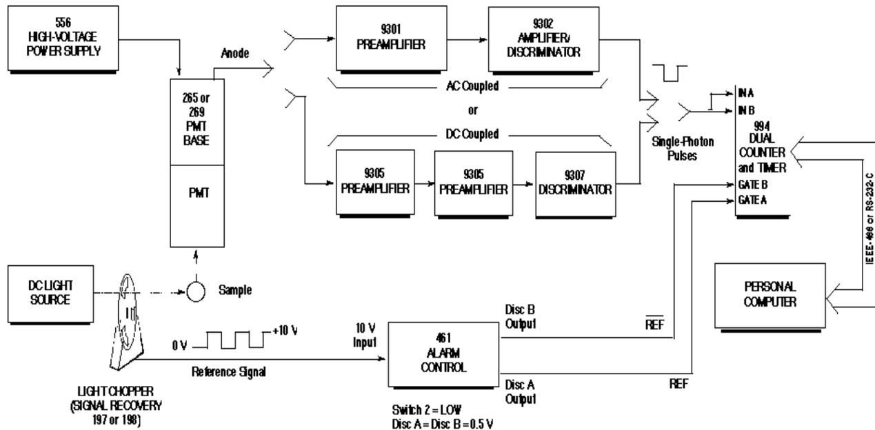
Fig. 3. Electronics for Single Photon Counting with a Light Chopper.
