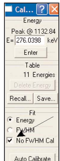
Fig. 15. Make Sure "NO FWHM Cal" is Marked.
