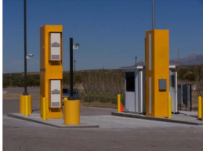
Figure 1 Installed HPGe Portal at Anthony, New Mexico
