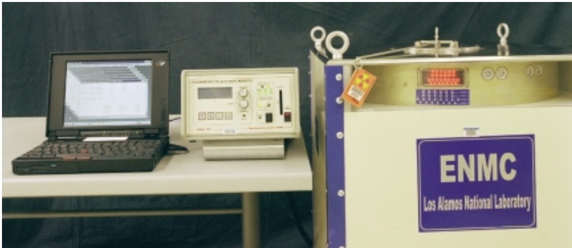
Figure 12. Photograph showing the integrated, operating ENMC/AMSR/INCC system components, left-to-right, a laptop PC running INCC version 4, a commercial AMSR (AMSR-150), and the ENMC.
