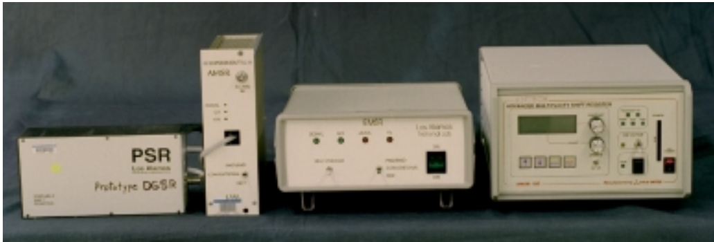
Figure 5. Photograph showing evolution of the Advanced Multiplicity Shift Register (AMSR). Left to right: the Dual-Gated Shift Register (DGSR), the Experimental AMSR (test-bed), the EMSR, and a commercial AMSR (AMSR-150)
