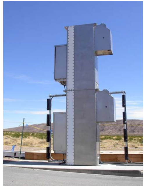
Figure 1 Prototype Cargo Portal on test site. Photo courtesy of National Nuclear Security Administration/Nevada Site Office
