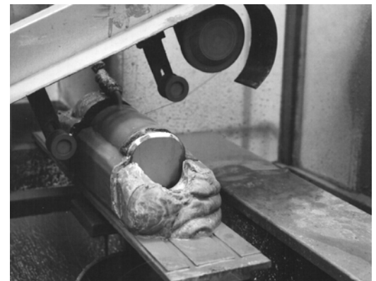
Fig. 6. A Mounted Crystal Being Sliced.
