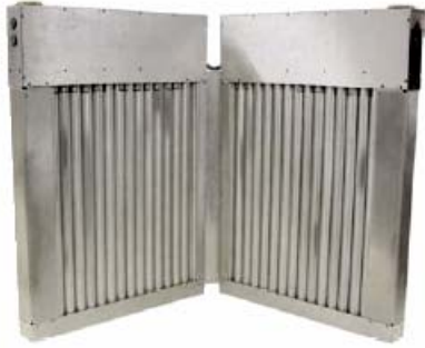
Figure 3 Instrument hardware showing 3He tubes
