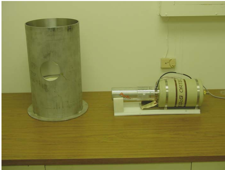
Figure 2. Detector viewing a HEPA filter in a Pad 19 filter housing at a source-to-HEPA centerline distance of 12 inches.
