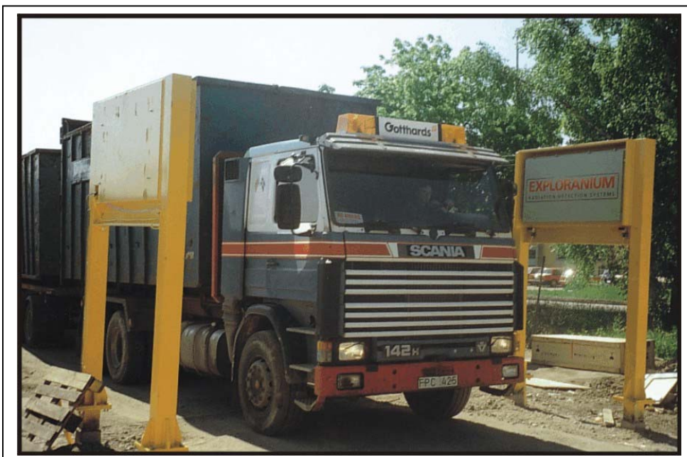
Fig. 2: AT-900 truck monitoring systems as normally used for scrap monitoring.
